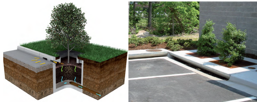
Figure A.2 Example of Tree Pits
