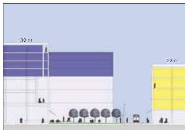
J: Street Section: Main Square and Cross Street Street width 38.5m, Tallest building height 30m Street width to building height ratio 1:0.78
