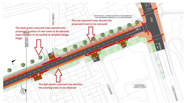
2. Extract from Preliminary Design Drawing sheet 5 of 11 – Section from Roundabout at Ashfield to Drogheda Street
