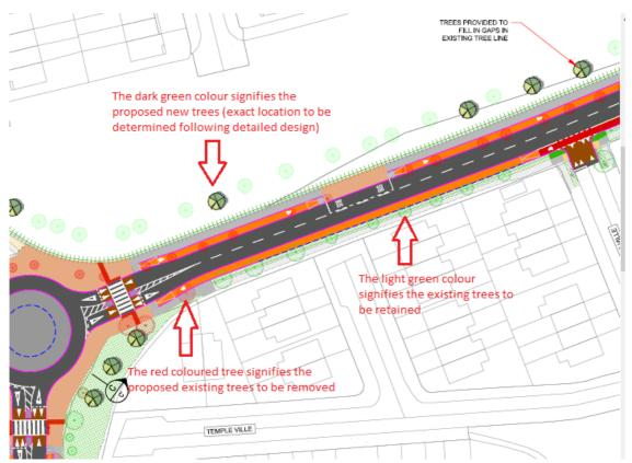
1. Extract from Preliminary Design Drawing sheet 3 of 11 - Section from Roundabout at Ashfield to Drogheda Street
