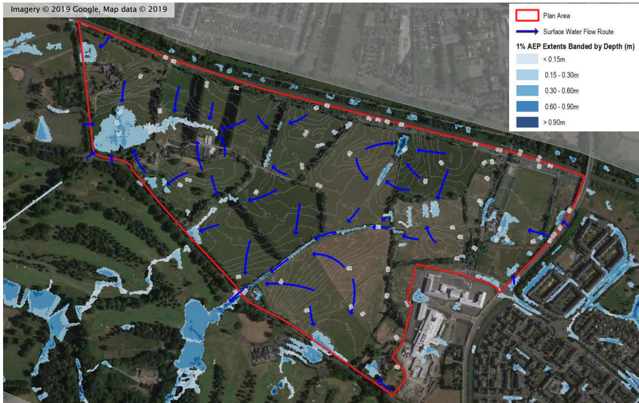
Figure 6-9 1% AEP Event Flood Routing
