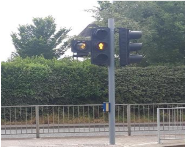
Holywell R125 – Signals Upgrade – Amber Countdown Timer for improved pedestrian safety
