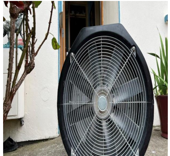
An air tightness test fan - used to determine the level of uncontrolled air flow through gaps or cracks in the fabric of a house.
