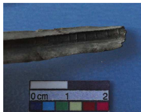
Fig.8. Detail of came 17E0302:19:6 showing reeding from milling process.
